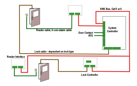
The following diagrams breaks the connections into these blocks:
