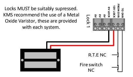
An emergency over-ride switch can be fitted that disables the power to the lock regardless of the access control system. The wiring for an emergency over-ride switch depends on the type of lock being used:
