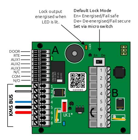
**Note:** Due to space considerations on the PCB, terminations are labelled 1 through to 8.
