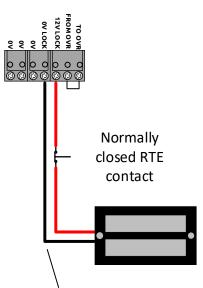
Example showing RTE breaking +12V to lock
