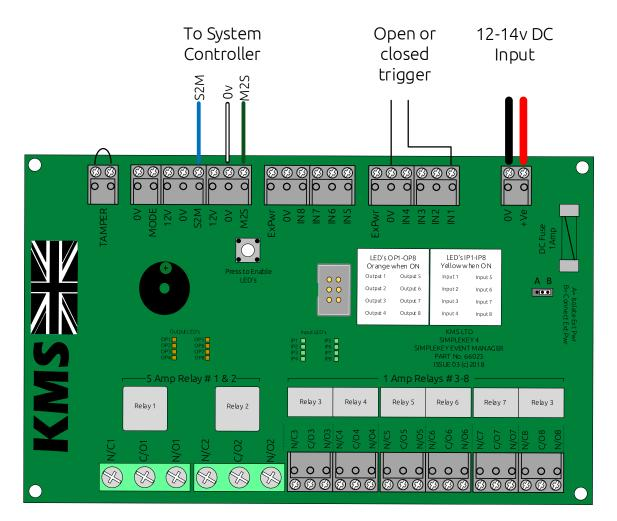
Volt free output relays. Relay 1&2 5Amp 240v Relay 2-8 1Amp 12v
